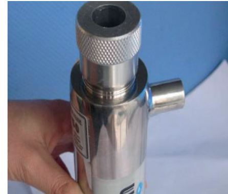
4. Tighten the big aluminum nut to the chamber
